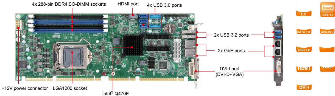
ROBO-8115VG2AR-Q470E is based on Intel® Q470E chipset and workstation processors. Built with flexible PCI express expansions, ROBO-8115VG2AR-Q470E is suitable for Medical, Industrial automation, and Digital Signage application.
